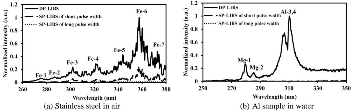
Fig. 2 Measurement results of stainless steel in air and Al sample in water under different conditions.
