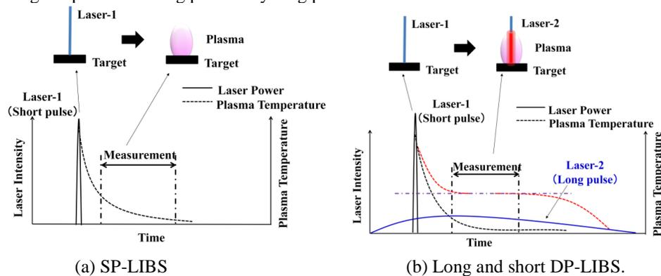
Fig. 1 Laser-induced plasma processes of single-pulse LIBS (SP-LIBS) and long and short DP-LIBS.
