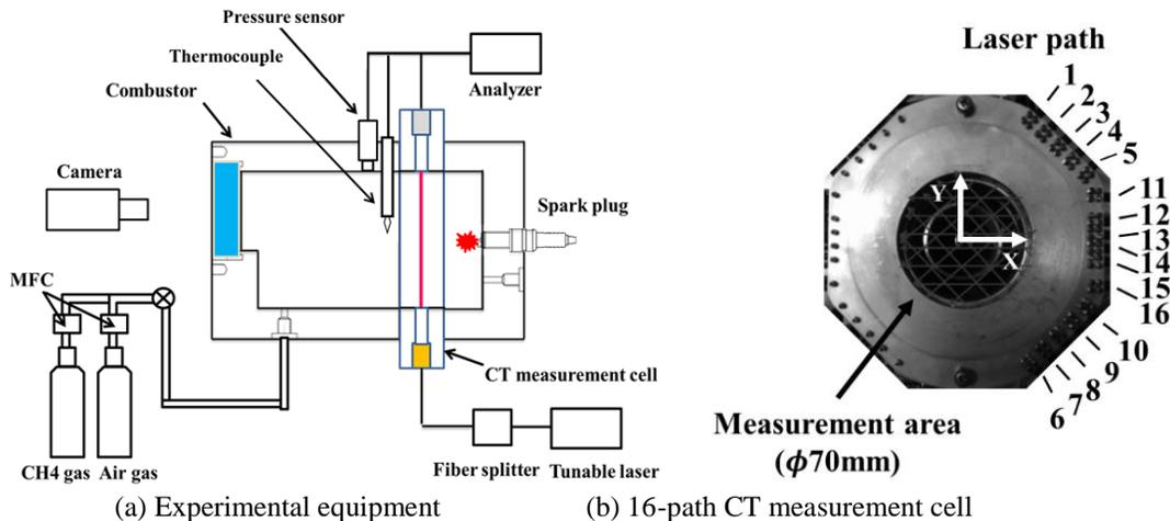
Fig. 3 Experimental apparatus of high pressure constant volume combustor measurement
