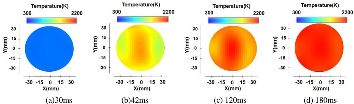
Fig. 5 Time series 2D temperature distributions measured by CT-TDLAS.
