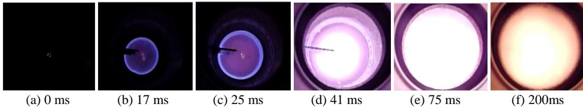
Fig. 4 Photographs of high pressure flames
